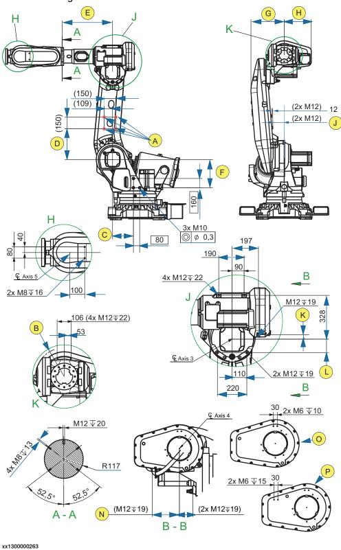
A Allowed position for attachment holes, M12 through. Be careful not to touch the cables when drilling.
